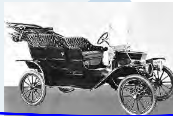
Ford Model T, combustion engine, 20 HP, in 1910
