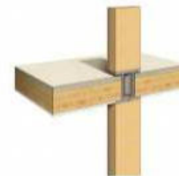
partial encapsulation during construction
