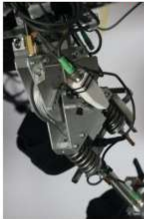
Schematic overview of bowden cable driven series elastic actuator
